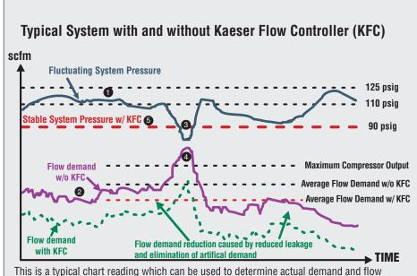
pattern in existing systems. Pressure **1** and flow **2** are inversely related, as can be seen at **3** and **4**. Pressure drops below the desired system pressure of 90 psig at **3** because the system cannot deliver the needed flow from storage at point **4**. The Kaeser Flow Controller reduces the flow demand in the system while maintaining stable system pressure **5**.
